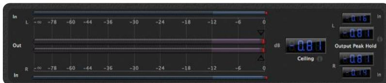
The four horizontal LED bar displays show the relevant peak values in the process. Click on any of them to reset the peak values.
