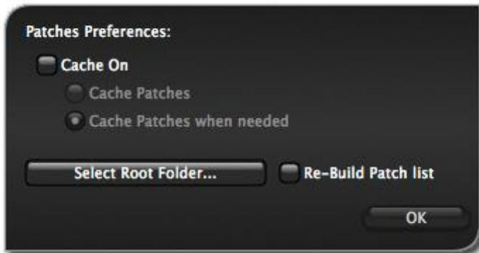
**Cache On:** allows you to activate the loading of all the presets in memory, so that the system doesn’t have to read from disk each time a setting is used. This is helpful to reduce the time of reading to disk.
